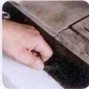
Open the air and damper valves completely.
